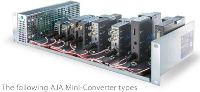
The following AJA Mini-Converter type can be installed in the DRM:
